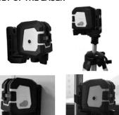
Set up the instrument as upright as possible to allow the self-levelling system to function within the range.
